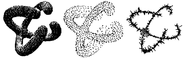
Figure 3: A continuous shape, a sampling of its boundary and the corresponding approached skeleton.
